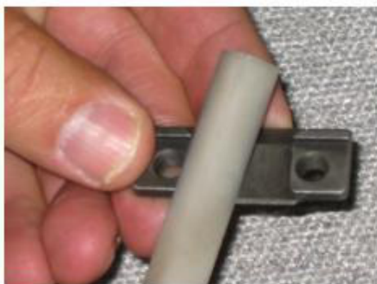
Hand polishing cutter blade with a fine stone.
