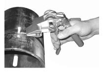
2. With ratcheting action, tension the band until clamp is tight. If necessary, band may be repositioned be releasing tension with levers.
