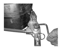
Roll tool over as far as tool will go, and push forward cutter handle. Remove tool and tap down ears of clip to complete clamp.
