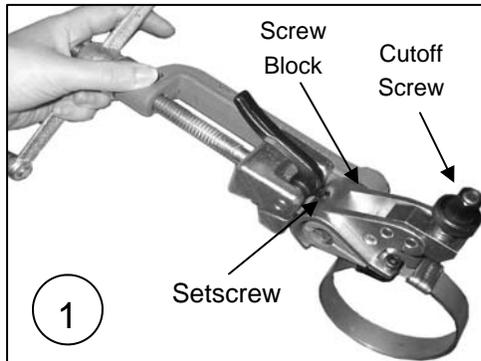
Place Heavy Duty Adapter on nose of BAND-IT Tool, positioned as shown. Cut-off screw should not extend beyond bottom of screw block. Line up tool and adapter slots and tighten two setscrews. Insert BAND-IT Junior or Junior SID clamp tail into adapter nose through all slots and grip end with band gripper lever.
