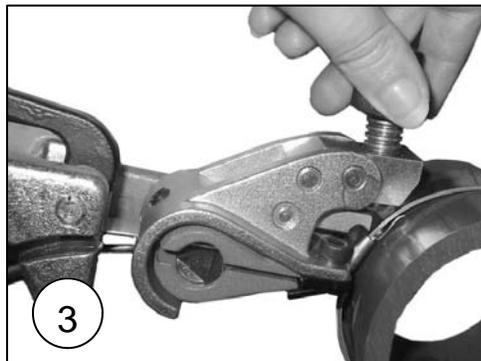
When properly tensioned, roll tool over hose, backing off tension handle  $\frac{1}{4}$  to  $\frac{1}{2}$  turn only, through course of rollover, (depending on type and size of hose) until shear hook grips buckle edge. Tighten knurled nut by hand, securing buckle tightly between edge of hook and nose of adapter.
