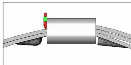
The finished BAND-IT Junior SID clamp lip lock will be bent upward 90° and have a cut-off edge (shown in green) that is flush to the edge of the buckle. Edges shown in red with hash marks are too high or too low and may result in lower lock strength or sharp edges.
