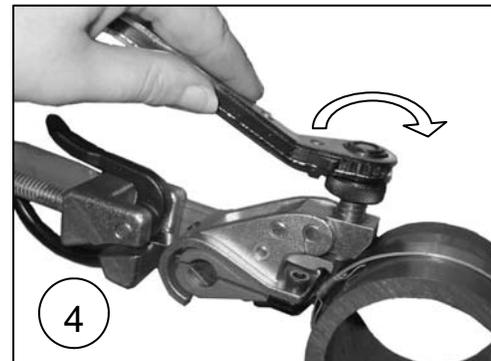
Place ratchet wrench on hex nut. Operate wrench clockwise until clamp is sheared. Clamp is now locked and completed.
