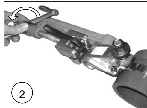
Install clamp over hose assembly. Tension clamp by turning handle of BAND-IT Tool clockwise.
